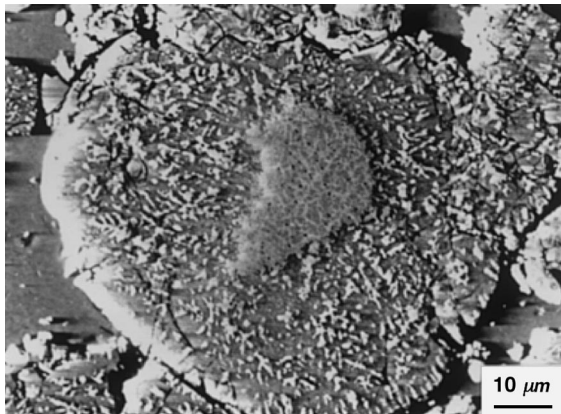
Fig. 8. Microstructure of the 9 wt% Nb fuel meat after 2 h at 500°C.
